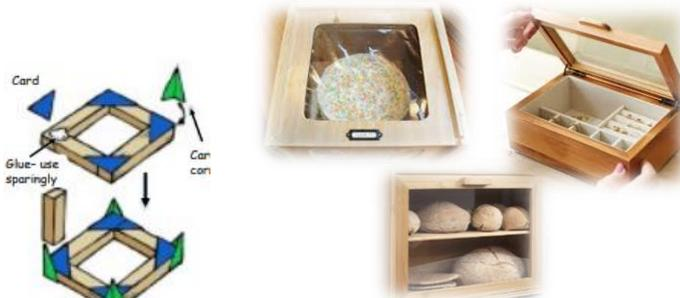
Creating triangles in your structure can strengthen it and make it more stable. There are different ways of doing this. You could glue card triangles to join two pieces of wood together, or use another piece of wood, paper or a plastic straw to connect two corners together.
